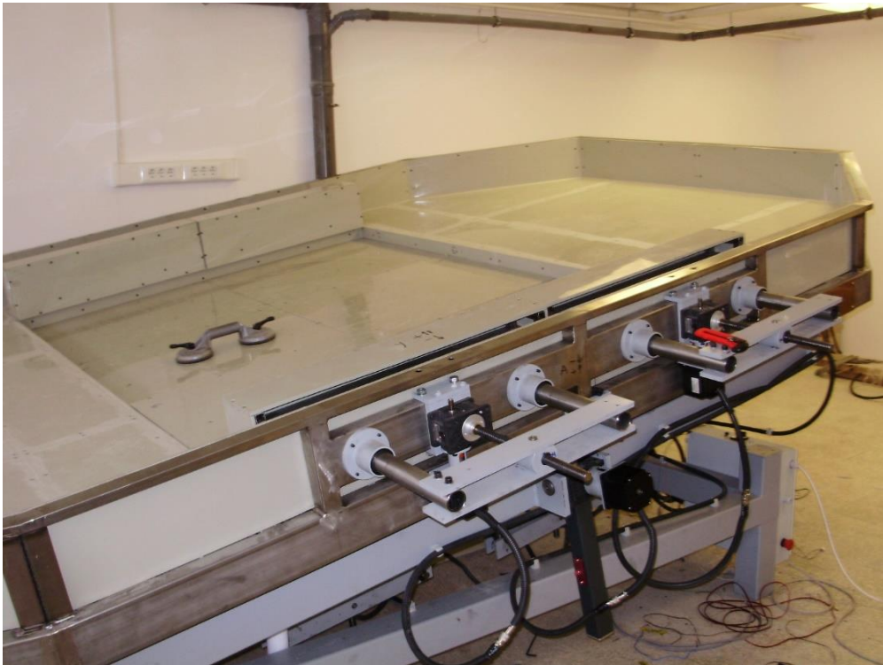
Figure 1.: The sand table with no experimental material inside. The vertical tectonically plates are clearly visible (in the middle of the table with a handler on the top of them). There are horizontal tectonic plates on the left and right side of the table. There are two electric engines on the left side (black boxes with silver rings).
